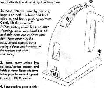
Blade Assembly Pront Release Back Release
